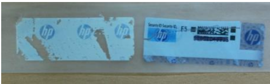
Figure 13: Adhesive left behind on product (left) and signs of tampering on label (right) on previous label
