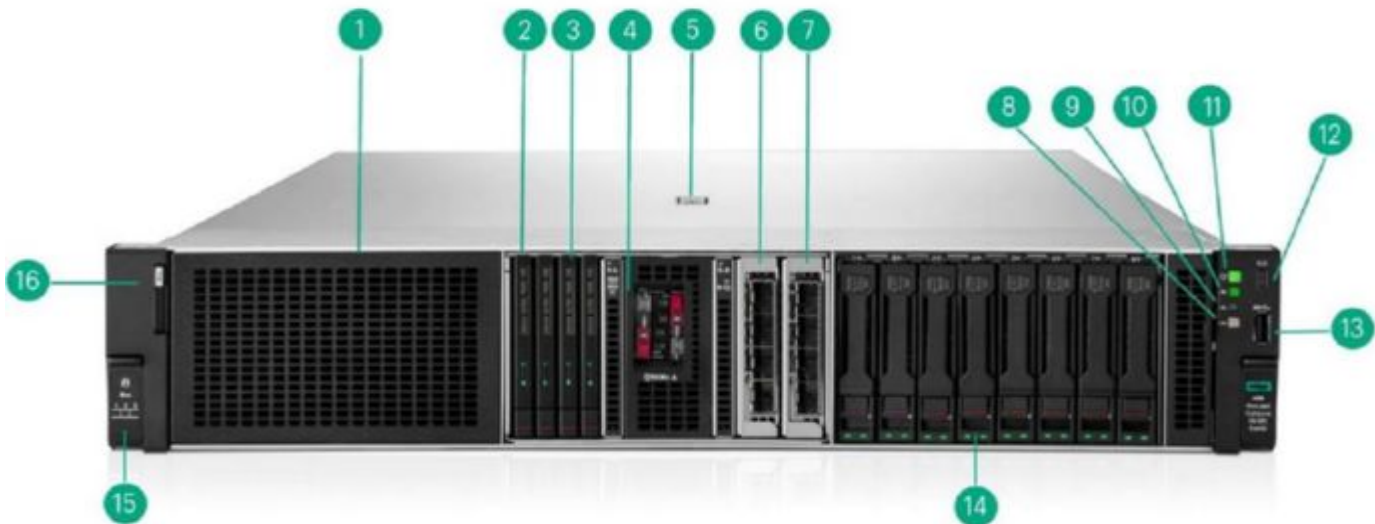
Front View -SFF CTO Server with optional multi-purpose cage
